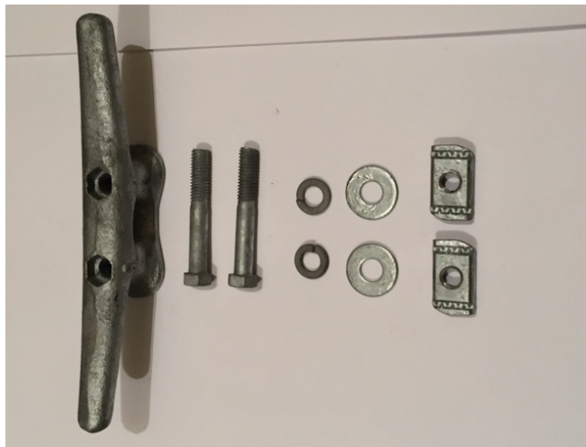
Method #1 Cleat and hardware for the aluminum track install
